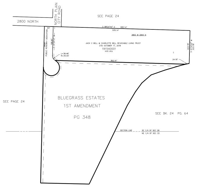
15' UTILITY & DRAINAGE EASEMENTS EACH SIDE OF PROPERTY LINES AS INDICATED BY DASHED LINES EXCEPT AS OTHERWISE SHOWN.
